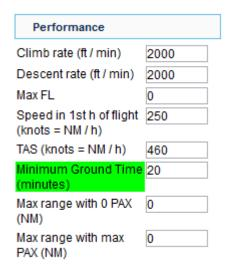
Once it is set, when you add a new trip and the difference between STA of the last leg and STD of the new leg is less than 'Minimum Ground Time', Leon will display a warning (see example below).
